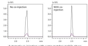
Automatic co-injection with water matches mobile phase conditions, preserving peak shape for early eluters
